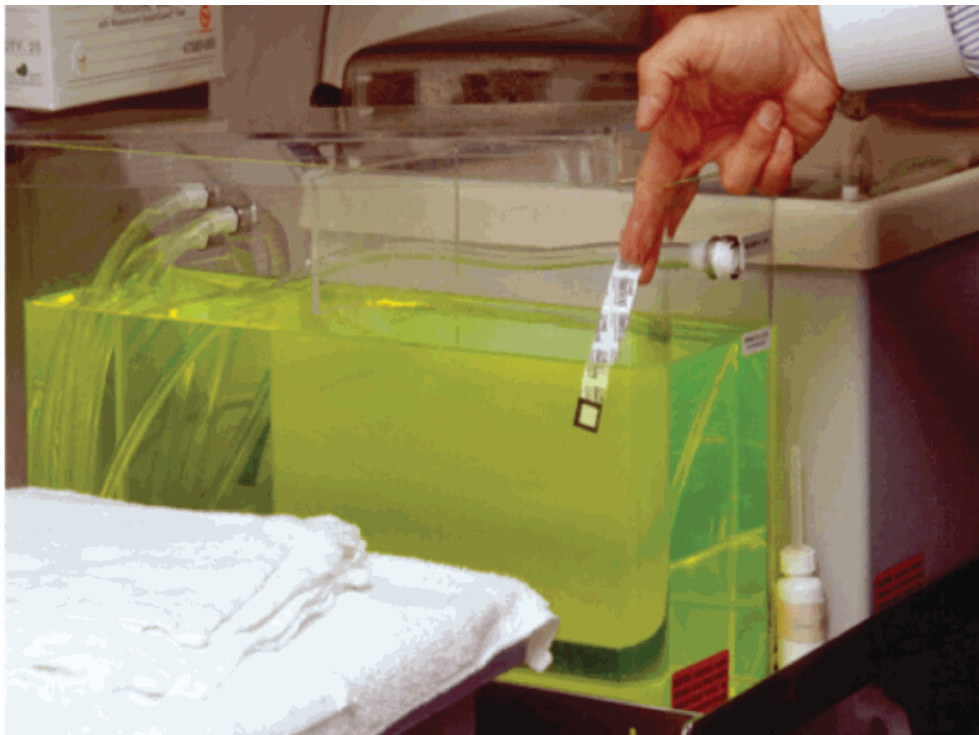
FIGURE 8-2: Testing the Disinfectant with Test Strip
